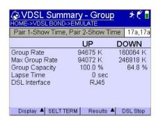
Figure 2. Show Time for bonded pairs requires that both pairs of a bonded group are active
