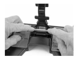
2.4 If using the 3M<sup>™</sup> Fibrlok<sup>™</sup> Assembly Tool 2501, rotate the toggle arms for the appropriate fiber size.
