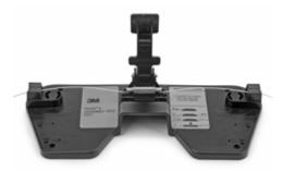
4.9 Pivot the handle of the 3M<sup>™</sup> Fibrlok<sup>™</sup> Assembly Tool 2501 down until it contacts the cap of the Fibrlok splice. Squeeze the handle of the assembly tool as shown in order to close cap and actuate the splice. When possible, secure the tool to a work surface for added support. A snap sound will be heard when the splice is actuated.
