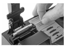
Note: Push fiber <u>straight</u> into fiber alignment guide, <u>NOT</u> AT AN ANGLE.
