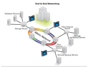
Thanks to end-to-end network testing capabilities, EXFO's FTB-860 enables fast deployment and configuration of Fibre Channel networks. Communication between the transport network, interconnection devices and end nodes can be validated with features such as BER testing, latency measurement, buffer-to-buffer credit estimation and port login capabilities.
