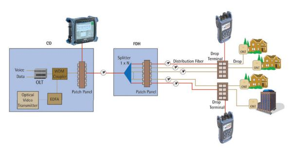
The FOT-930 allows for automated, bidirectional loss and ORL testing of passive optical networks (PONs) at 1310 nm, 1490 nm and 1550 nm, the three wavelengths recommended by the ITU-T (G.983.3) for PONs.
