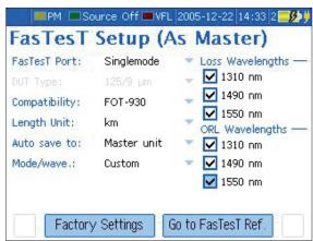
While performing FasTesT measurements, the FOT-930 can launch automated loss and ORL measurements on all three wavelengths and perform fiber-length measurements.
