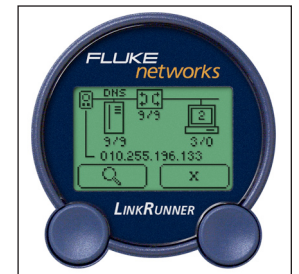
Ping DNS server or key devices, and observe response time.
