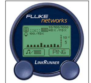
See device capabilities, actual link speed, and utilization levels.
