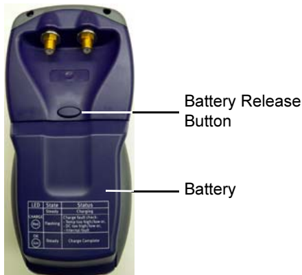
Figure 1 Back of DSAM Meter
