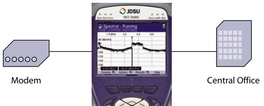
Example of HST-3000 performing Spectral Monitoring
