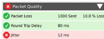
Identify if packets are being lost over the RF portion of the data layer
