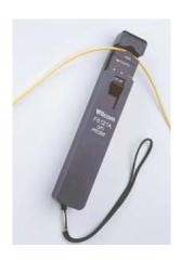
The Wilcom OFI Model F6121A Probe is a rugged, hand-held, easy-to-use maintenance and installation instrument that identifies optical fibers by detecting the optical signals that are transmitted through a singlemode fiber. The F6121A utilizes non-destructive macro-bend detection, which eliminates the need to identify a fiber by opening it at the splice point. Thus, the probability of interrupting service is eliminated.
