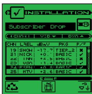
Pressing the “cycle” soft key provides more detail by bringing up a list of all channels. Passing channels have a “3” in the right hand column.
