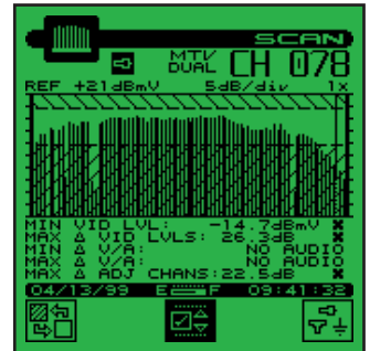
The Full Scan display shows all user-defined video carriers. The unique limit check feature quickly checks the results against user-defined analog and digital limits.
