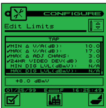
Limit sets for analog channels and a limit set for digital channels.
