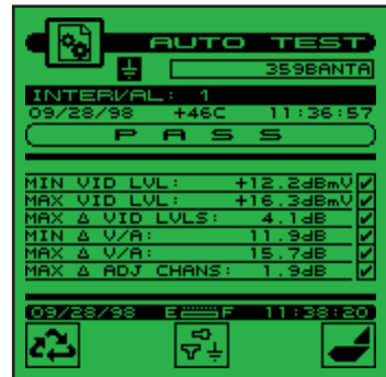
Auto Test results are time, date, and temperature stamped and can be stored, viewed, printed, or uploaded to StealthWare™ software.
