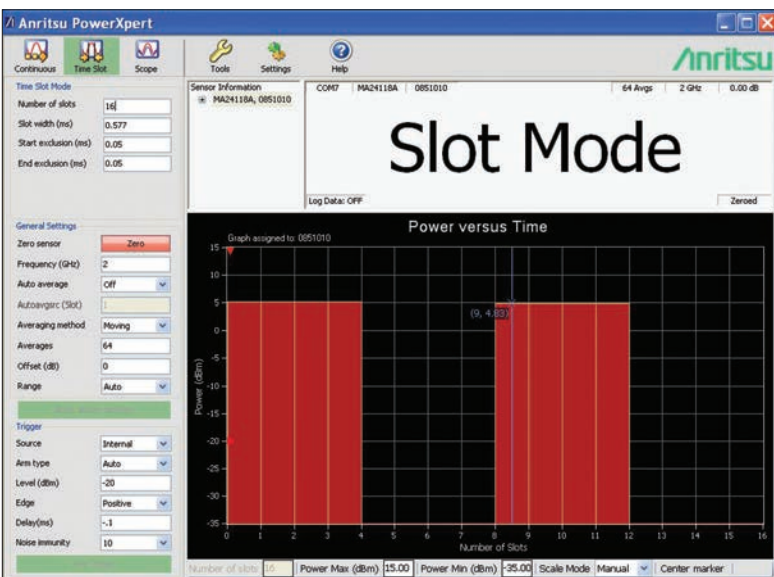
Measurement of a GSM four slot waveform with a MA24118A and PowerXpert in Time Slot mode
