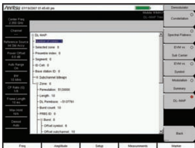
DL MAP screen displays the DL MAP zone information in a decision tree format.
