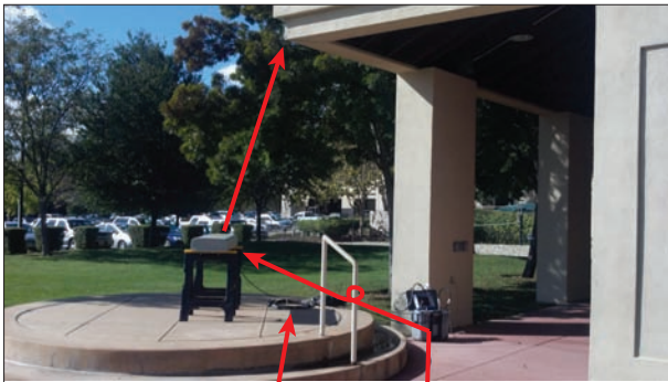
Locating multiple PIM occurrences in antenna cables with DTP
