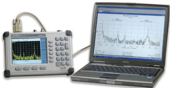
Connect Site Master to a PC via a serial (null modem) cable to transfer data or further analyze results
