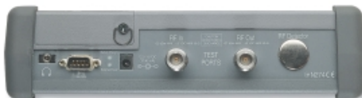
Panel connections include a 9 pin D-sub RS-232, precision test port connector, DC power input, headphone jack and an optional RF detector connection for the power meter operations.
