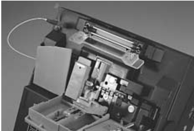
Model M90 Splicer with new electrode flap design, heat-shrink oven and pigtail adapter
