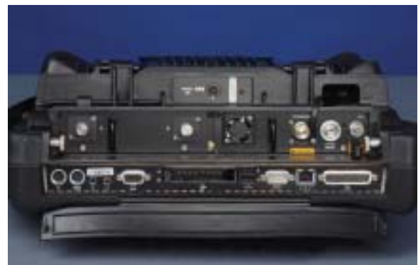
Optical Multitester - Rear View with OTDR Module | Photo TEQ27
