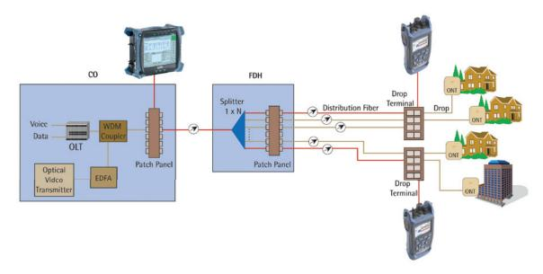
The FOT-930 allows for automated, bidirectional loss and ORL testing of passive optical networks (PONs) at 1310 nm, 1490 nm and 1550 nm, the three wavelengths recommended by the ITU-T (G.983.3) for PONs.
