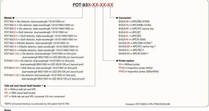
a. Connector type for the talk set is the same as the one specified for the main source.
