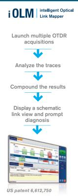
Using a unique and patented automated multipulse and multi-wavelength acquisition approach, the field-proven iOLM surpasses the traditional OTDR and linear view for expertlevel link characterization of any fiber network.
