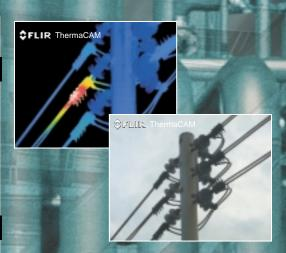
The ThermaCAM PM 695 is the first IR predictive maintenance camera to provide both thermal and visual imaging in one system.
