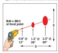
Use the Fluke 66 within 5 m (15 ft.) of the intended target. At greater distances, the measured area will be larger (approximately the distance divided by 30).
