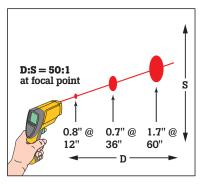
Use the Fluke 68 and 68IS within 8 m (25 ft.) of the intended target. At greater distances, the measured area will be larger (approximately the distance divided by 50).
