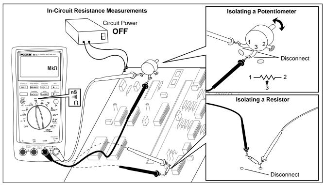
Figure 3-5. Resistance Measurement
