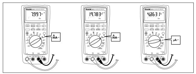
Figure 3-11. AC Current Measurement
