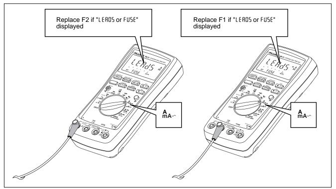
Figure 6-1. Testing the Current Fuses
