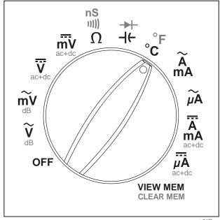
Figure 2-2. Rotary Switch
