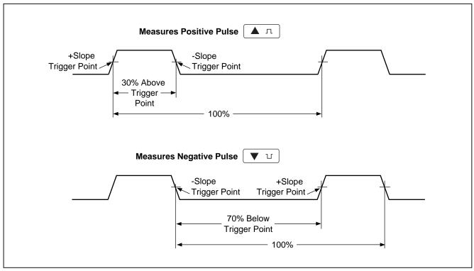
Figure 3-15. Duty Cycle Measurements
