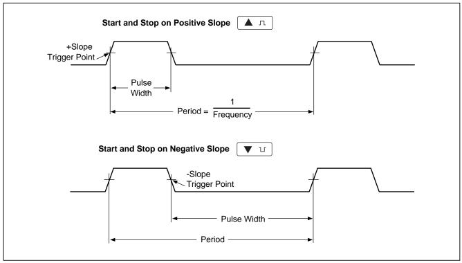
Figure 3-17. Pulse Width Measurements
