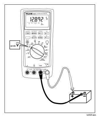
Figure 3-4. DC Voltage Measurement
