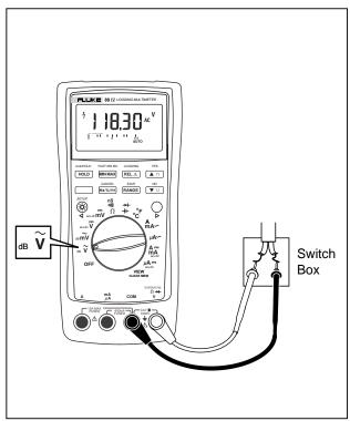
Figure 3-1. AC Voltage Measurement
