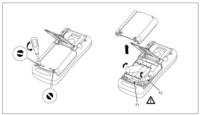
Figure 6-2. Battery and Fuse Replacement
