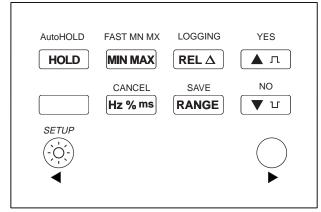
Figure 2-3. Pushbuttons
