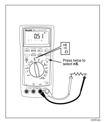
Figure 3-7. Conductance Measurement
