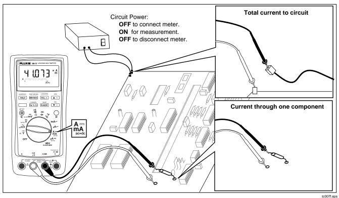
Figure 3-12. DC Current Measurement
