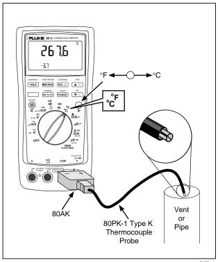
Figure 3-10. Temperature Measurement
