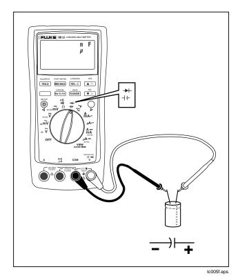
Figure 3-8. Capacitance Measurement
