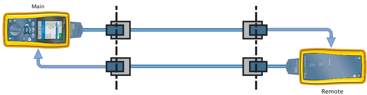
Figure 4: Alternate method for Alien FEXT measurement when testing horizontal cabling and a separate communication link is not available.
