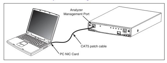
**Figure 5. Direct Management Port Connection**
