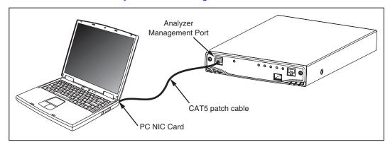
**Figure 5. Direct Management Port Connection**
