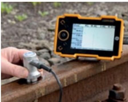
The USM Go has been designed to provide flaw detection capability in inspection situations throughout the industrial and process spectrum, from aerospace to power generation and from the automotive sector to the oil and gas industry.
