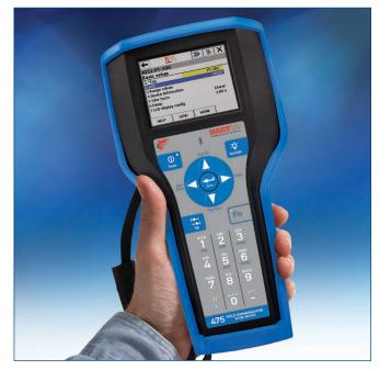
The 475 Field Communicator is designed to support all HART and FOUNDATION fieldbus devices from all vendors.
