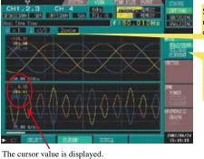
Select a waveform display range of 2, 4, 10, or 12 cycles.
