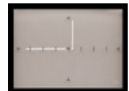
The ON state of the SCR shows a diode signature as the device is triggered
