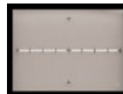
The OFF state of the SCR shows an open signature
