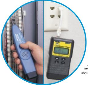
The Tone Mode generates four different tones on all pairs, a selected pair, or selected pin. The tone signal has constant tone amplitude over the life of the battery and two tone amplitude of normal and half (HI on pair and Low on pin).
