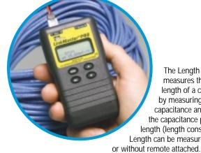
The Length Mode measures the length of a cable by measuring its capacitance and using the capacitance per length (length constant). Length can be measured with
