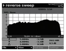
Tight reverse sweep points are setup in the sweep plan to view better resolution of the entire return path. Helping to find mismatches or other problems heading back to the headend or hubsite.
