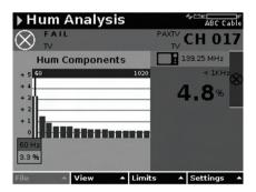
Undesired electrical interference can appear on a video channel as one or two horizontal bars. A Hum measurement reveals if any electrical interference is present on tested channel.
