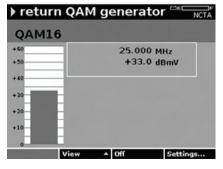
The Return QAM Generator eanables operators to test and prove upstream network performance.
