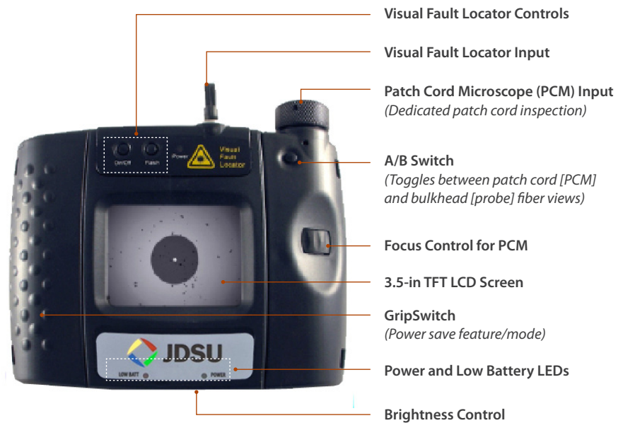
HD2-P4-V Display with Integrated Patch Cord Microscope (PCM) and Visual Fault Locator (VFL)
