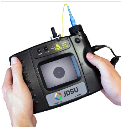
HD2-P4-V Display with Integrated Patch Cord Microscope (PCM) and Visual Fault Locator (VFL)
