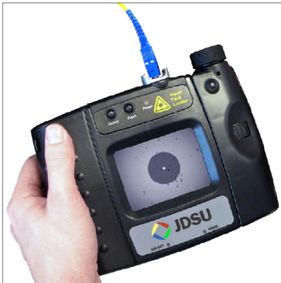
HD2-P4-V Display with Integrated PCM and VFL
