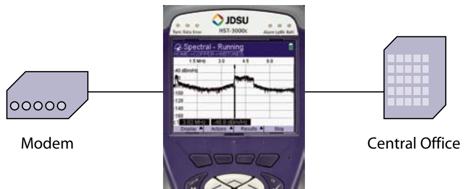
Example of HST-3000 performing Spectral Monitoring
