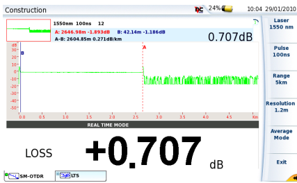
Figure 5 Real time mode -Total loss measurement
