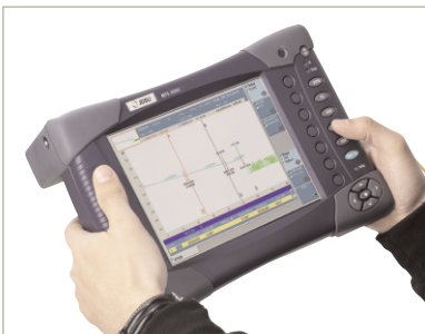
Figure 6 MTS/T-BERD 6000 platform with OTDR module
