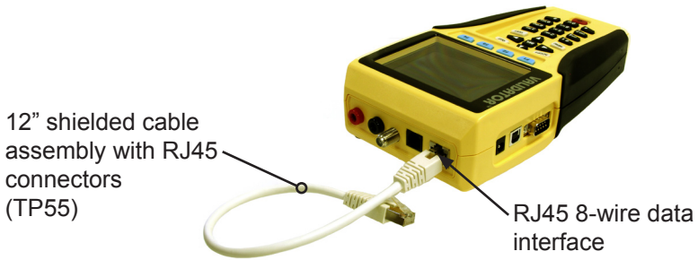
Figure 1. TP55 Connected to Validator
