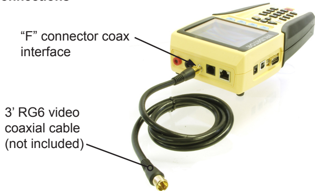
Figure 4. Video Coaxial Cable Connected to Validator
