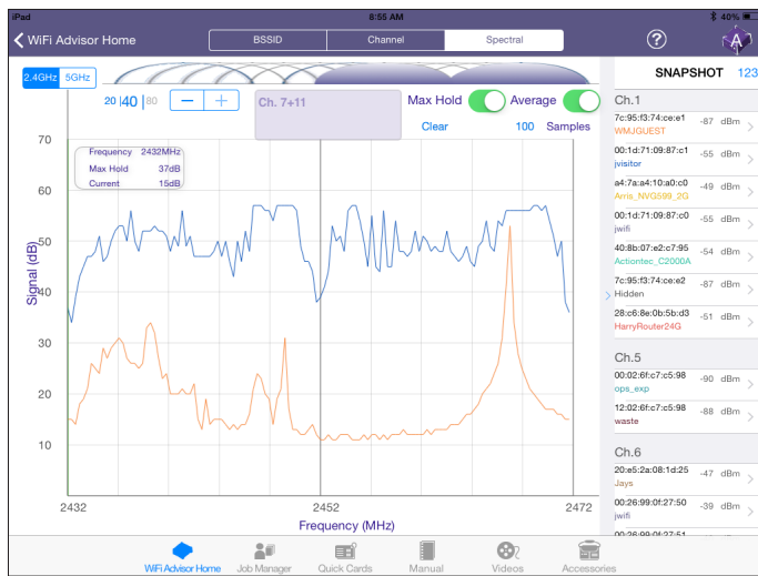
Spectral view shows interference within a channel
