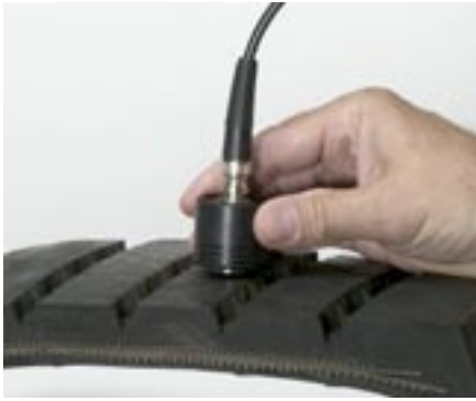
Measure depth to steel / ply cords in rubber conveyor belts or tires.
