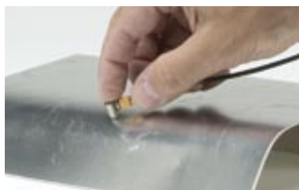
You can measure critical thickness metal thinning caused by bending.
