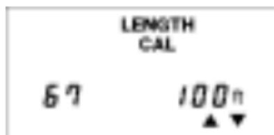
If you know a cable's NVP, change the displayed numbers using the ▲▼ keys until the appropriate NVP is displayed. The cable length will automatically adjust to the new NVP.
