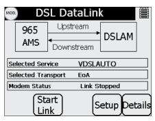
VDSLAUTO mode automatically connects at the the highest possible connect rate/service type (i.e. VDSL2, VDSL, ADSL2+)
