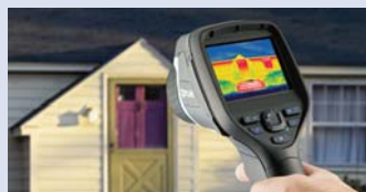
Infrared cameras quickly locate moisture related problems
