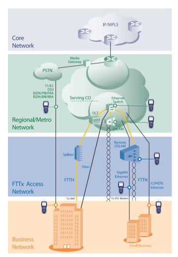
In enterprise networks, the HST-3000 tests DS3, Ethernet, and IP-based services such as VoIP in use by today's bandwidth-hungry businesses, enabling service providers to offer solutions and ensure service level agreements (SLAs) that match the growing demands of enterprise customers.
