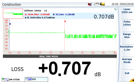
Figure 5 Real time mode -Total loss measurement
