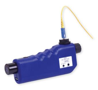
Inspect patch cords with NOYES VS 300 from AFL. Designed for field use, the VS 300 scope delivers a high quality end-face image at 400x magnification. Quickly identify scratches, dirt or other problems normally associated with poor network performance.
