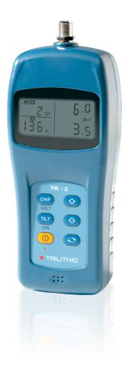
*Voltmeter mode* displays the battery voltage and trunk voltage (AC or DC).
