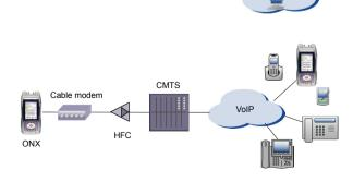
One Expert tests VoIP throughout the IP network registration with gateway, test calls on and off the network, and measures near- and far-end IP QoS and MOS.
