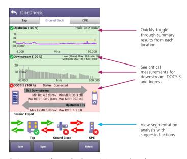
During any specific test, OneExpert simultaneously performs a powerful suite of additional tests in the background. By simply swiping through results, technicians can evaluate system wide performance including MER and BER across all channels, DOCSIS results (showing individual channel details), SmartScan results, and off-air ingress such as LTE carriers that are infiltrating the plant and causing problems.
