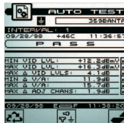
AUTO TEST results are time, date and temperature stamped and can easily be stored, viewed, printed (MS-1200D, MS-1300D, MS-1400) or uploaded to StealthWare software (MS-1300, MS-1400)
