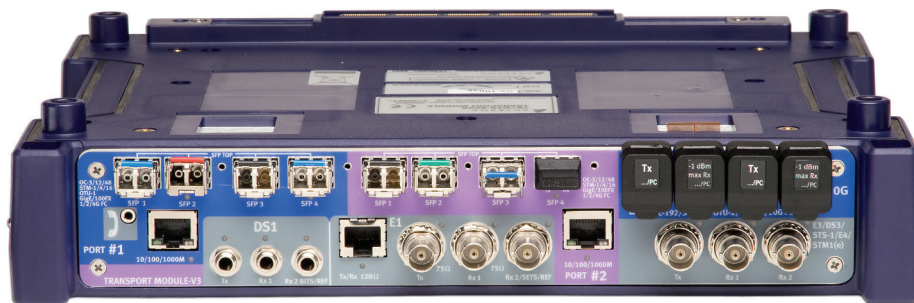
Port view of T-BERD/MTS-8000 Transport Module
