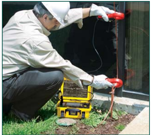
The Model 6471 performs a fast and easy way to measure the value of the earth/ground using the 2 Clamp method (no auxiliary rods needed).
