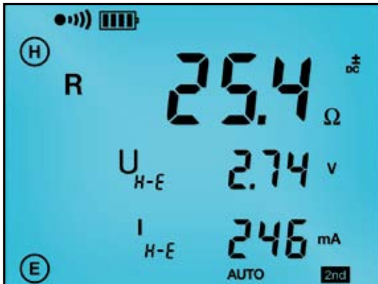
The 2-Point Bond test displays lead connections, bond resistance test results, test voltage and current.
