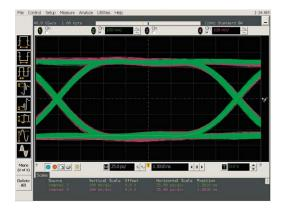
The industry's flattest frequency response leads to excellent correlation between scope only (green trace) and scope plus probe (red trace) measurements as shown in this dual infinite persistence eye diagram.
